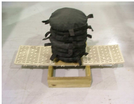
Test #2 Setup – 400 lbs
